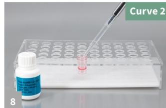
8 Add 700  $\mu$ l sample diluent to the red dilution cup and mix up and down 5 times
