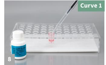
8 Add 700  $\mu$ l sample diluent to the red dilution cup and mix up and down 5 times. Continue to step 11.
