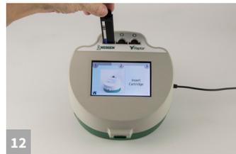
12 Insert cartridge into the Raptor reader. Select Curve 1.
