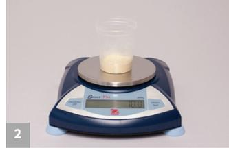
2 Obtain a representative sample. Grind and weigh out a 10 g sample
