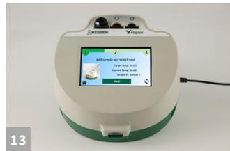
13 Add 400  $\mu$ l sample from the red dilution cup to the back of the Raptor cartridge. Reader will start automatically
