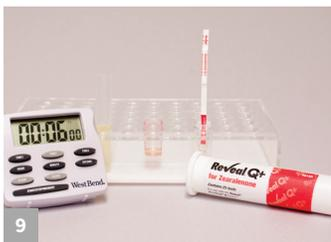
9 Place a new Reveal Q+ for Zearalenone strip into the sample cup. Set a timer for 6 minutes.
