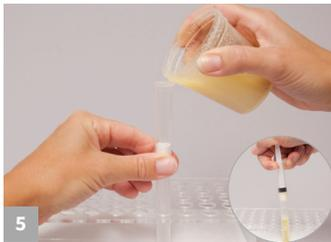
5 Allow to settle, then filter collecting a minimum 3 mL filtrate.
