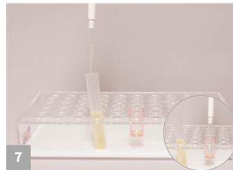
7 Add 100 µL of the sample extract to the red dilution cup and mix up and down 5 times.
