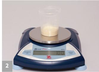
2 Obtain a representative sample. Grind and weigh out a 10 g sample.
