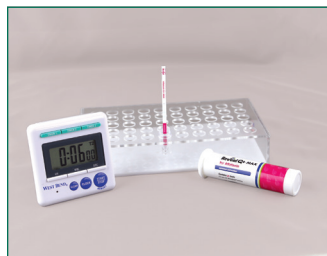
10. Place a new Reveal Q+MAX for Aflatoxin strip into the sample cup. Set a timer for 6 minutes
